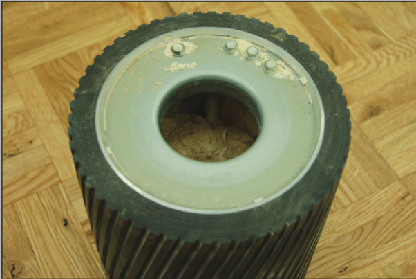
Pic. 9 Dust and debris in the drum
