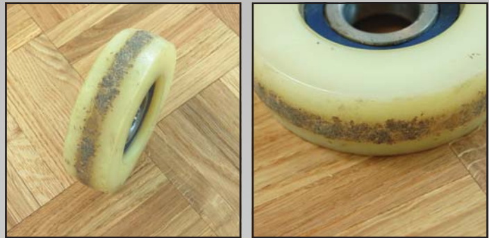
Pic. 4 and 5 Heavily soiled side wheel, new type
