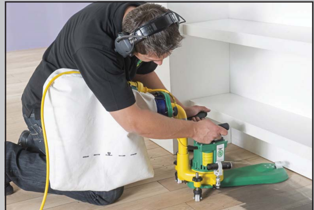
Pic. 6 The FLIP® with long attachment sanding under a built in shelf.
