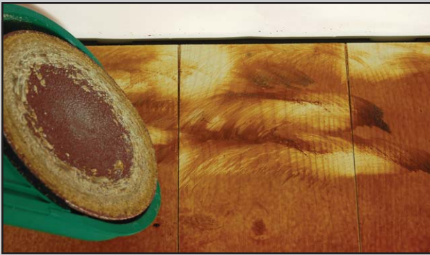
Pic. 2 Sanding a thick layer of lacquer with normal sanding material.
