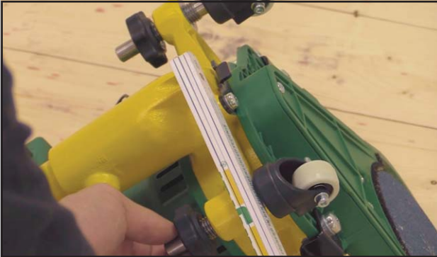
Pic. 9 Setting the FLIP® wheels with a ruler.
