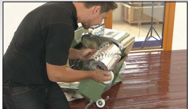
Pic. 5 Installing the milling drum on to the HUMMEL®.
