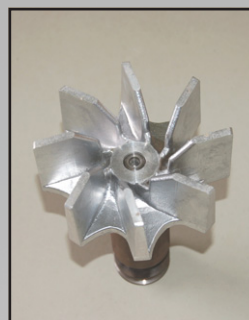
Pic. 5 / 6 Fan insert; latest design / old design; worn out
