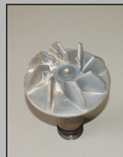
Pic. 5 / 6 Fan insert; latest design / old design; worn out
