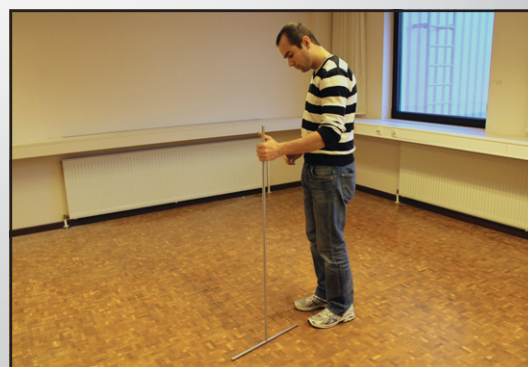
Pic. 6 Testing for loose pieces
