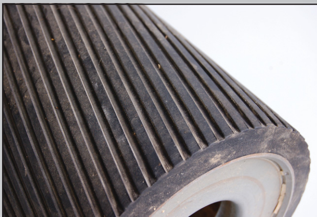
Pic. 12 Worn out sanding drum profile
