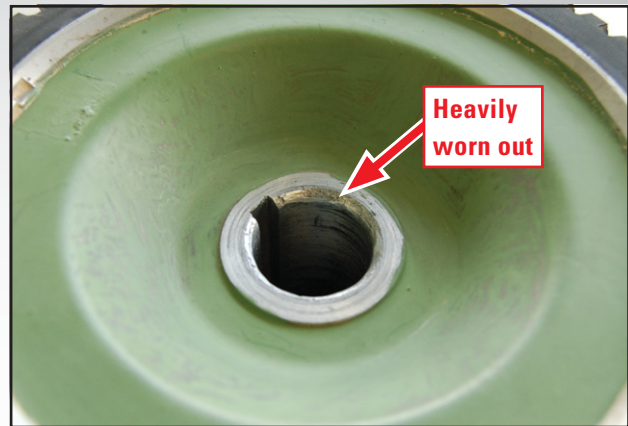
Pic. 10 Aftermarked / recovered drum with a worn out bore for the sanding shaft
